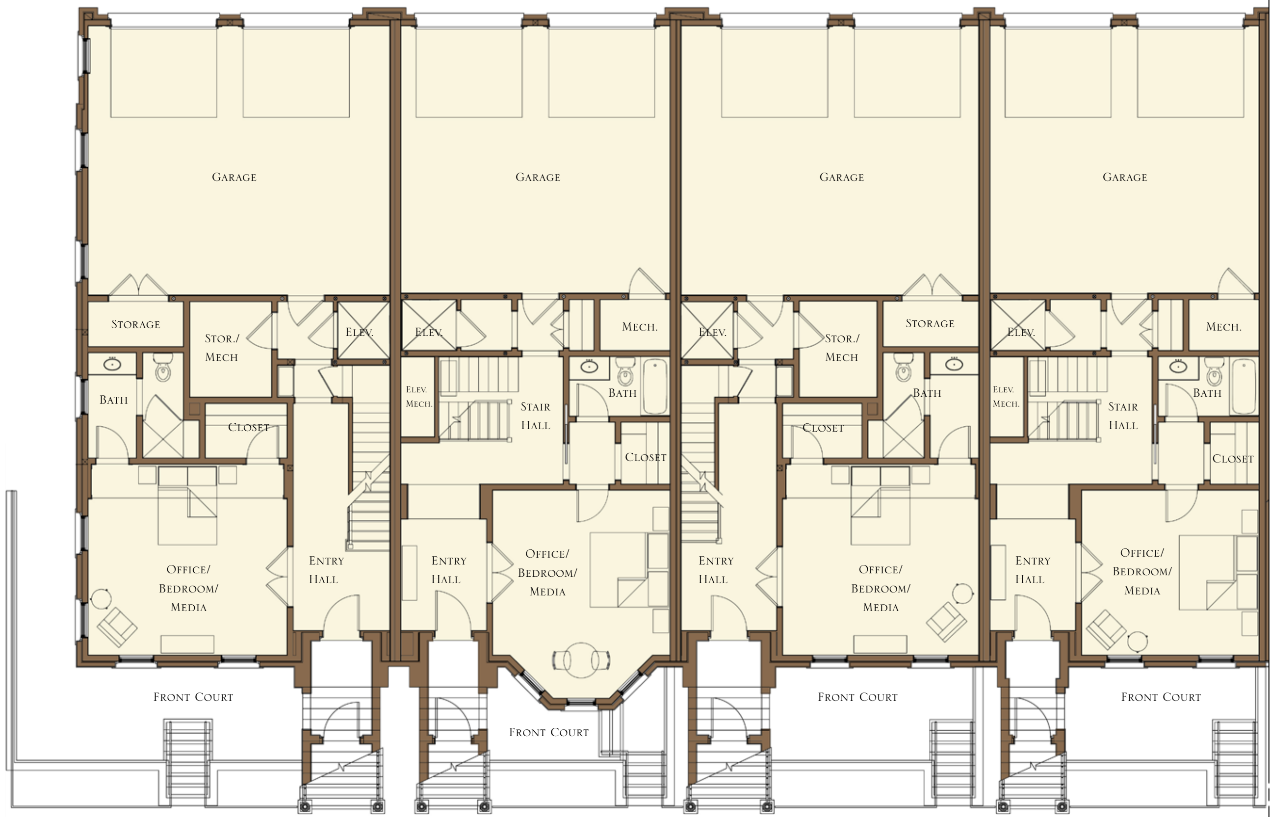
LOWER LEVEL FLOOR PLAN
